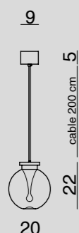
1593.1L SOSPENSIONE / HANGING LAMP Glass Ø20 cm - cable 200 cm LED 1 x 8,4W DIMM - 350 mA - 2700 or 3000°K CE IP20 Δ 1m
