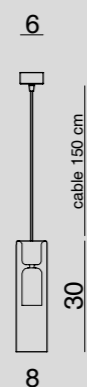
1383.1L SOSPENSIONE / HANGING LAMP Glass Ø8 cm - cavo/cable 150 cm G9 1 x max 42W 230V CE IP20 1m
